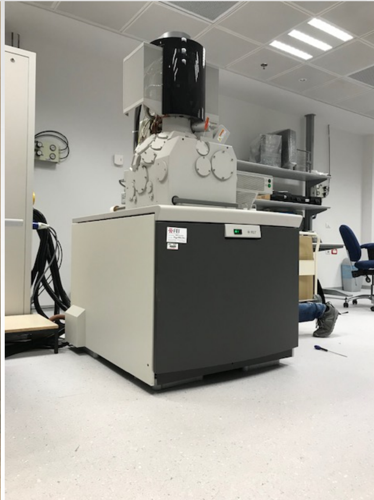
FEI Meridian SEM – ArisMD installed under the SEM
